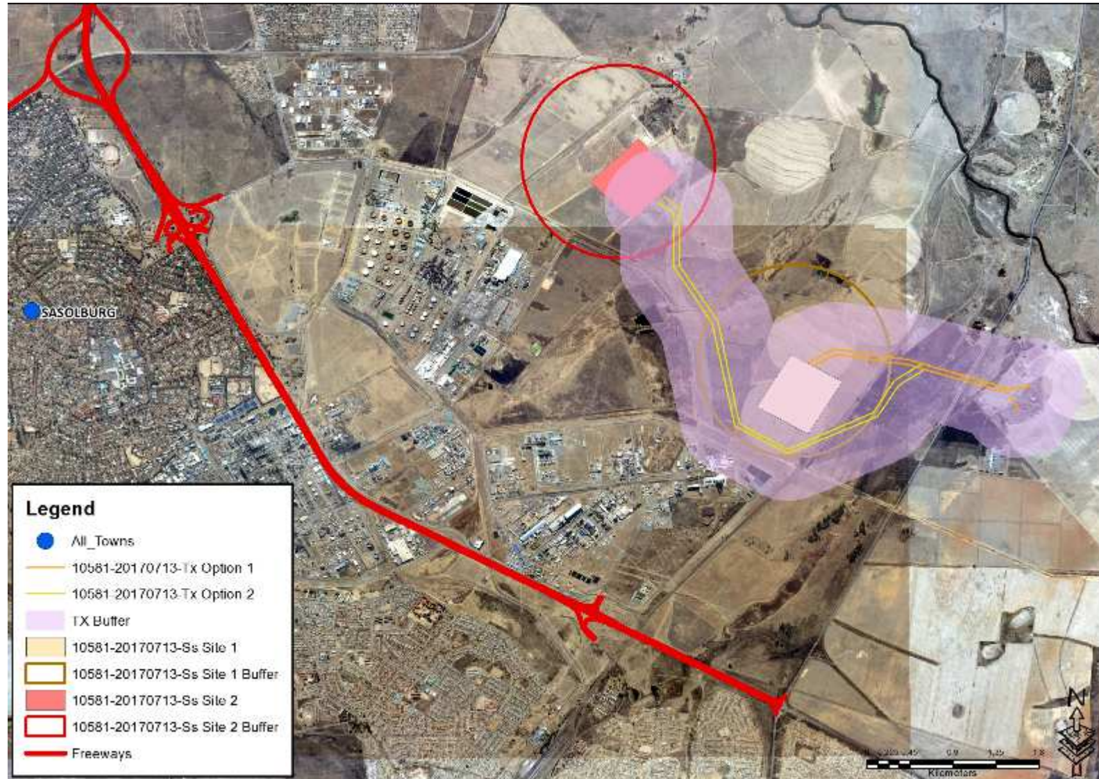
Figure 1: Proposed substation sites and associated power lines
