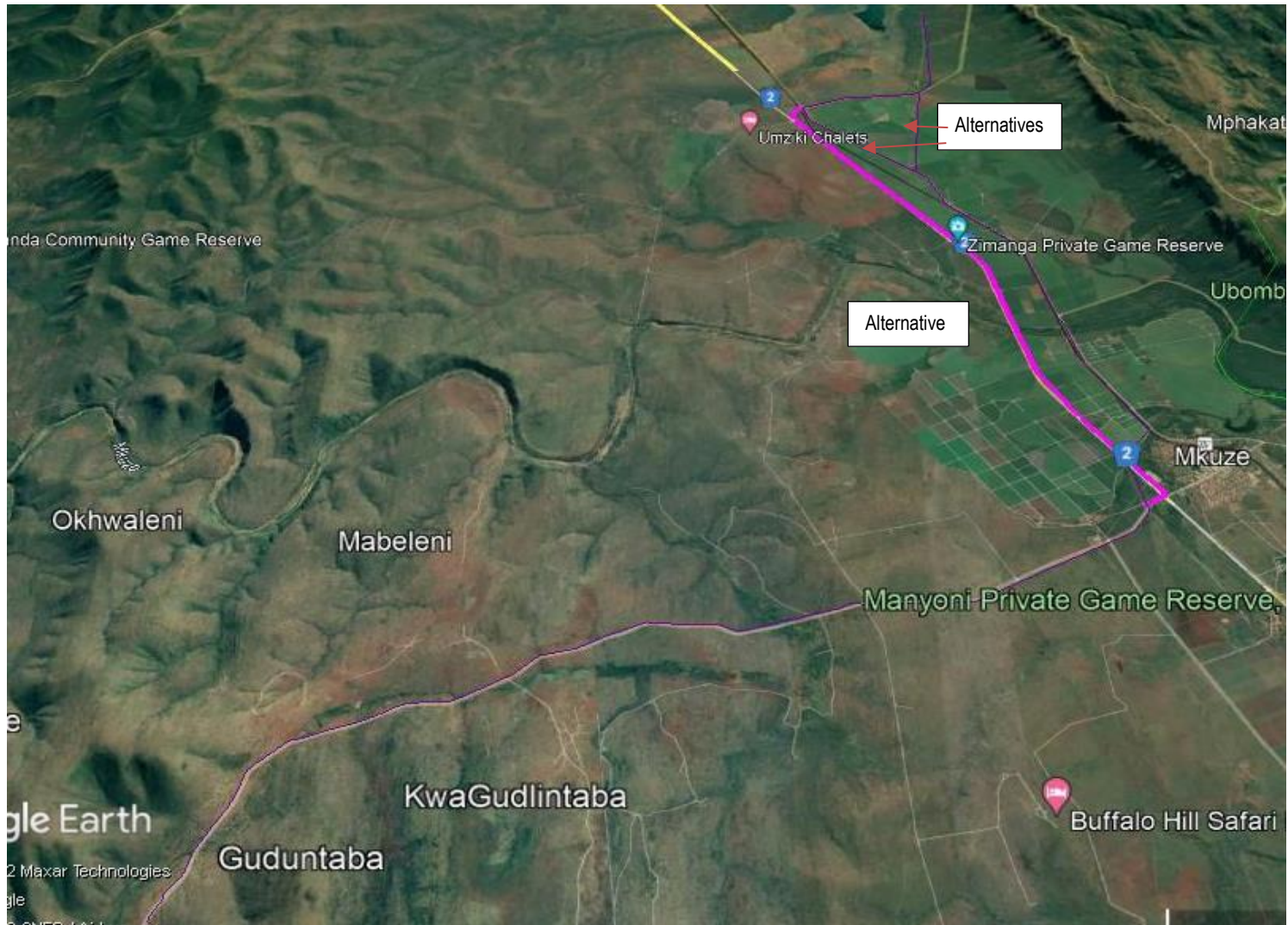
Figure 1: Bulk water pipeline indicated in purple with alternative route indicated in pink
