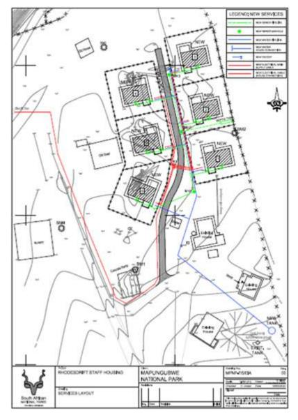
Figure 6. Proposed layout of staff houses with bulk services (Detailed drawings are appended in Appendix A)
