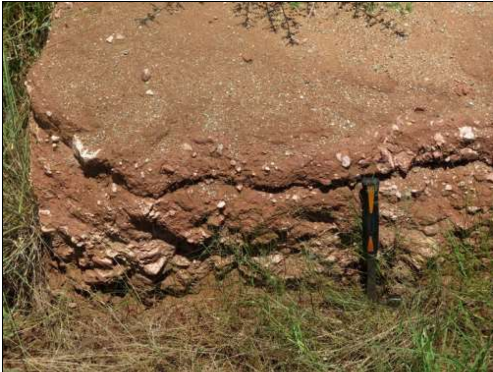
Figure 39. Sandy, well-consolidated soils with embedded rubbly calcrete gravel clasts, trench exposure at the Park Management Offices site (Hammer = 30 cm).
