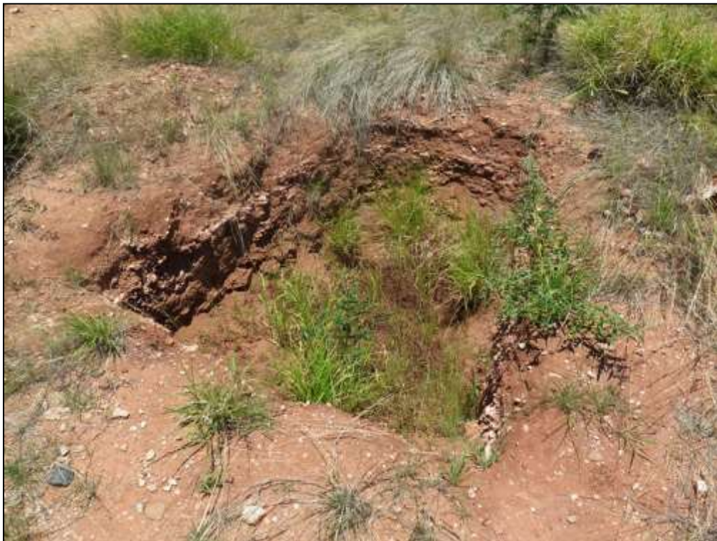
Figure 39. Sandy, well-consolidated soils with embedded rubbly calcrete gravel clasts, trench exposure at the Park Management Offices site (Hammer = 30 cm).
