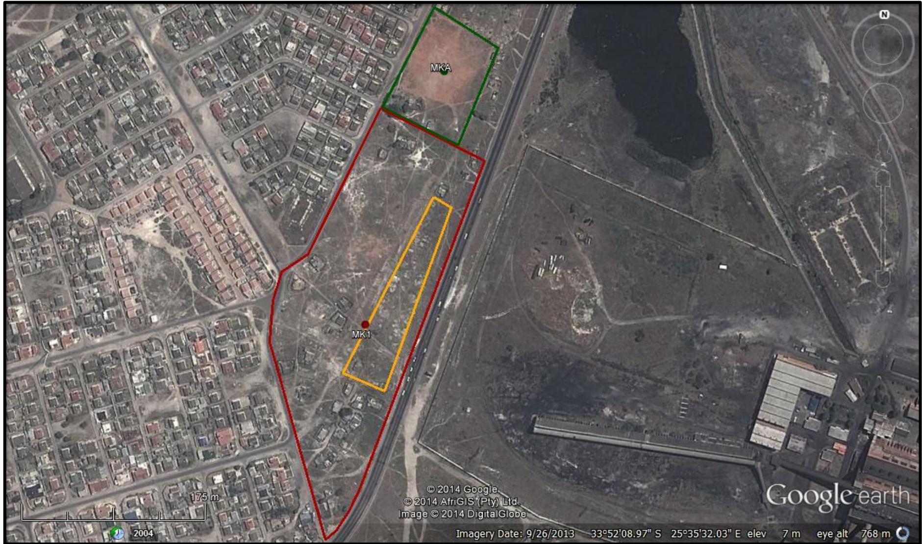
Figure 3: Close-up aerial view of the area proposed for the Masakhane Village Housing Project showing the general GPS points recorded, the additional area surveyed (green outline), and the occurrence of the remains of building foundations (orange outline).
