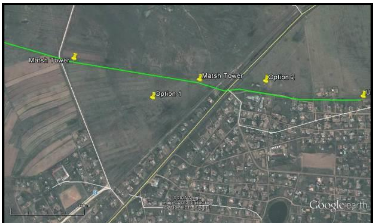
Figure 2. Google aerial photograph showing the location of the proposed substations and associated powerline routes.
