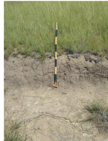
Figure 6. Residual deposits at the site consist of alluvial deposits of Quaternary age. The alluvial deposits are made up of grey and yellow sandy clays varying between 0.1 m and 2.0 m in thickness.
