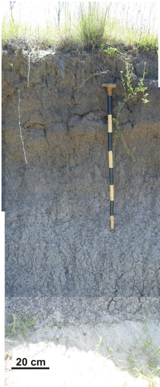
Figure 6. Residual deposits at the site consist of alluvial deposits of Quaternary age. The alluvial deposits are made up of grey and yellow sandy clays varying between 0.1 m and 2.0 m in thickness.
