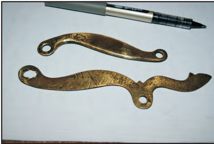
Figure 59: Sideplate from the collection of C. Shapiro. The roman numeral XII is an Ordnance assembly number. (Photo: Maitland 2010)
