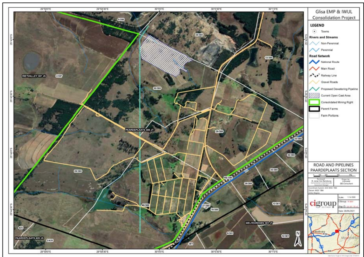
Figure 12:: Proposed Gravel Roads and Dewatering Pipeline in the Active and Planned Mining Areas.
