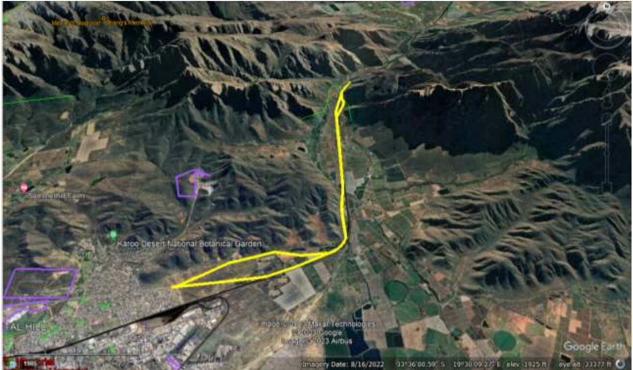
Figure 3. Option 2. A new alignment will run through existing farmlands, parallel to the existing railway until km 7. In the last section of the road a tie-in with the existing road will take place. Google Earth.
