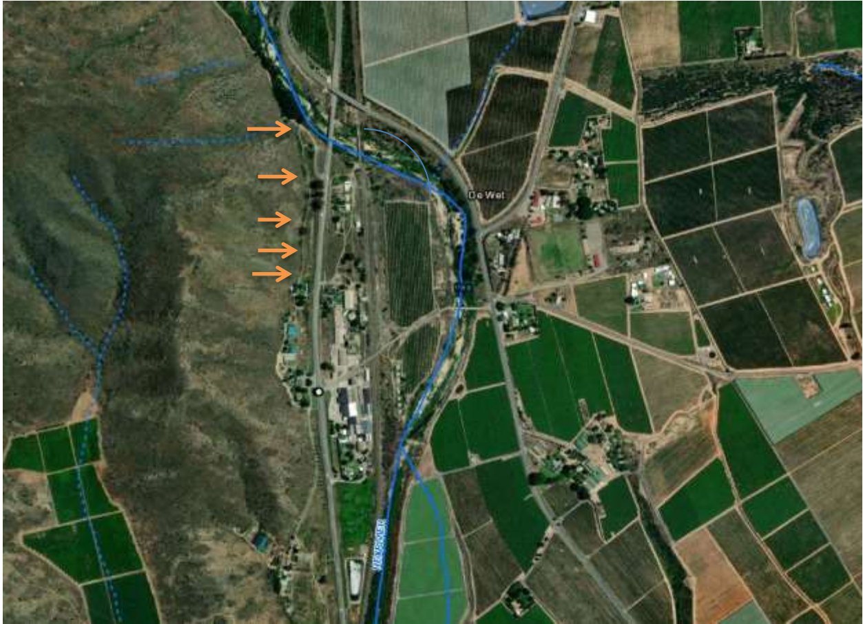
Figure 21. This figure shows the flow of water from the high mountains, down the valleys and into the Hex River. The pale orange arrows indicate the possible source of the water which drains into the irrigation ditch, and the path of flow of the irrigation ditch. The water may also originate from the close-by Hex River via an underground source. Source: Google Earth.
