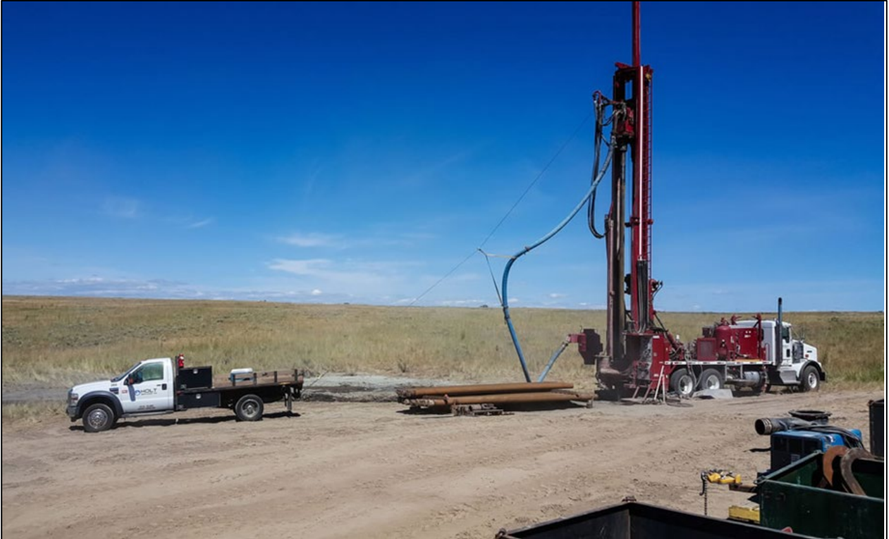
Figure 3: Example of the type of drilling rig to be used. Source: Basic Assessment Report Figure 4.
