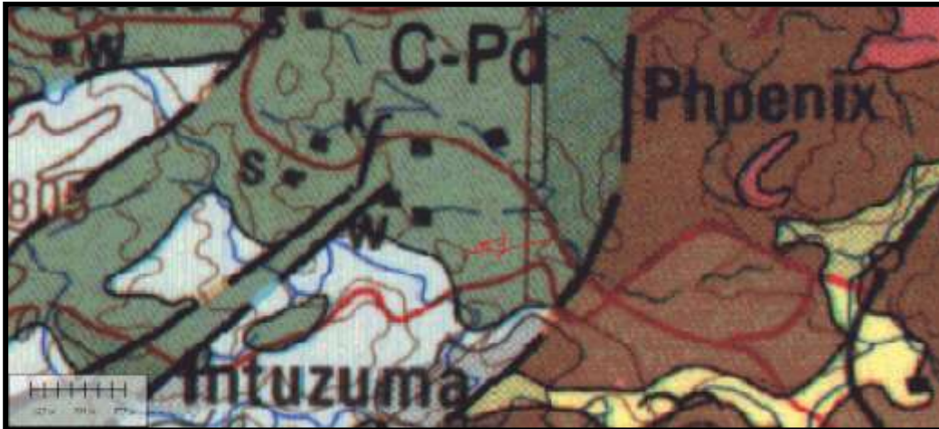
Figure 2 Geology underlying the sewer line is deeply weathered shale of the Dwyka Group
