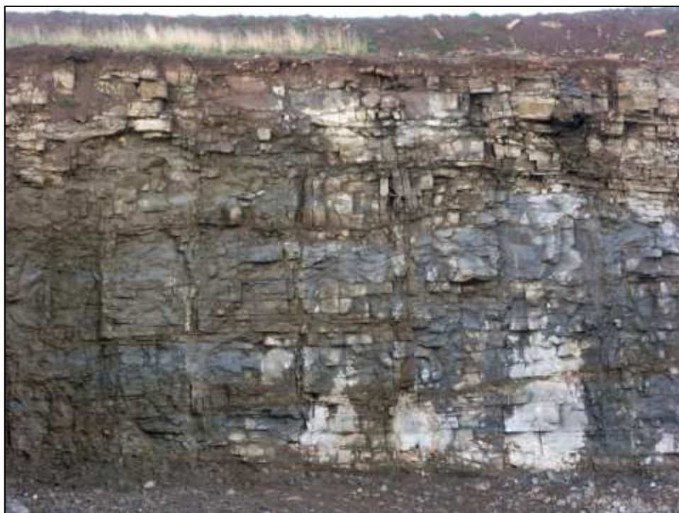
Fig. 13. Amalgamated grey, tabular sandstones of the Oudeberg Member, Balfour Formation exposed in the cut face of the Afrimat aggregate quarry on Klipfonteyn 150 (Loc. 239). Note gently-dipping erosional surfaces.
