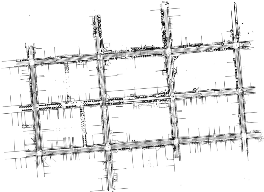
Topographical survey of the roads and sidewalks of the Operation Reclaim area – the basis from which the urban design work has followed.
