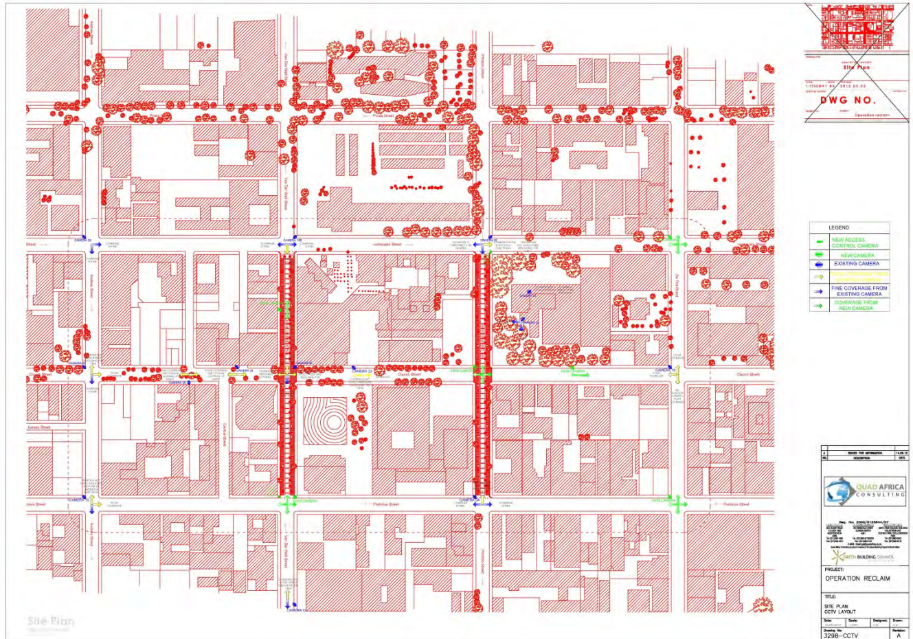
The survey of existing CCTV camera positions.
