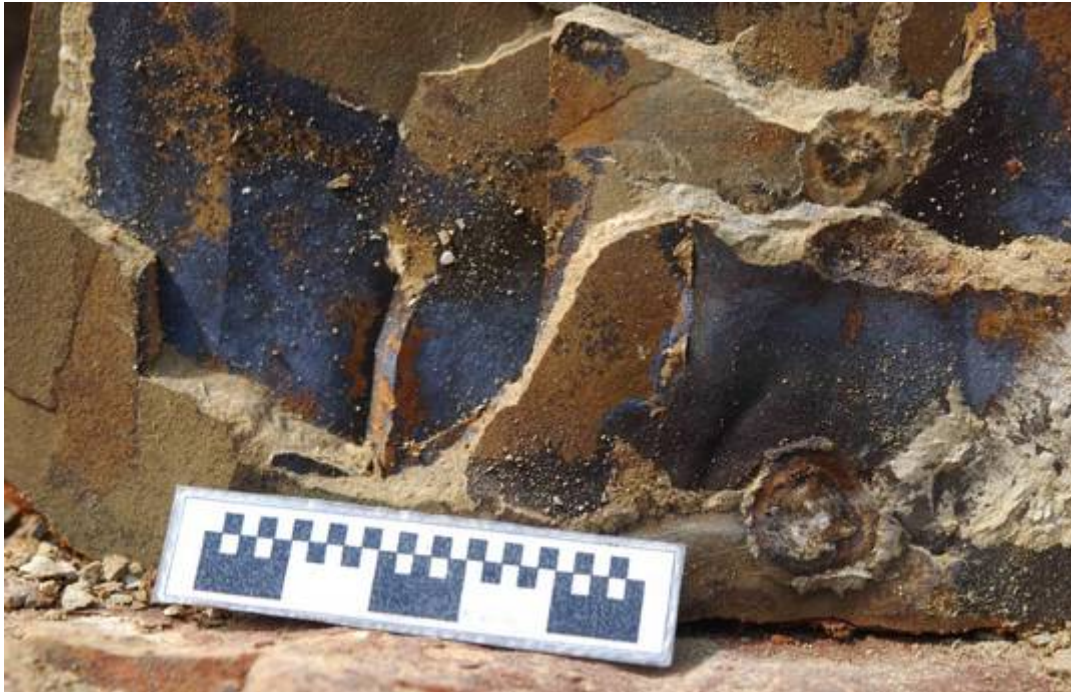
Figure 8: Thermally altered sedimentary derived rock which provides the source of aggregate at borrowpit 2.
