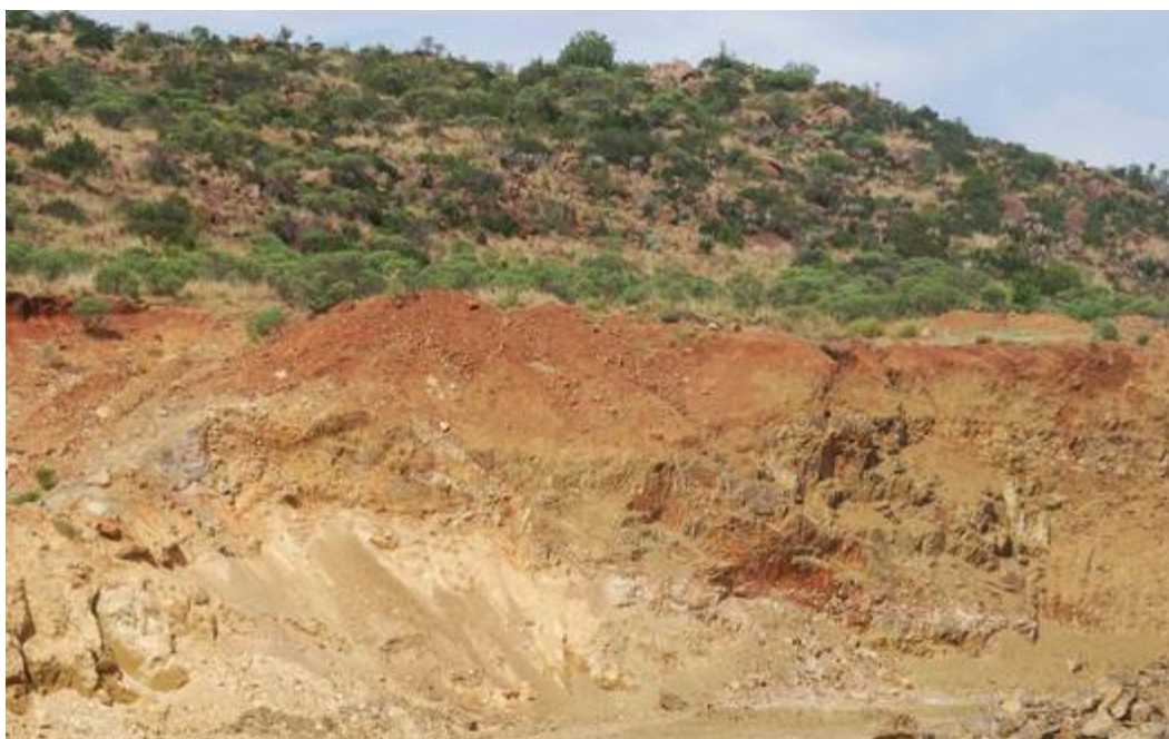
Figure 7: Borrowpit 2 showing a wedge of thermally altered sedimentary rock in the foredound at right, underlain by pale weathered dolerite in the foreground at left. A dolerite comprised ridge is visible in the background.
