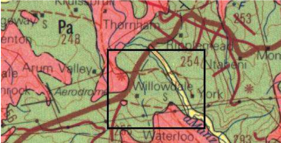
Figure 3: Extract from the Kokstad 3038 1: 250 000 Geological Map. Grey (Pa) is the Estcourt Formation and red is Karoo Dolerite. Aproximate area boxed.
