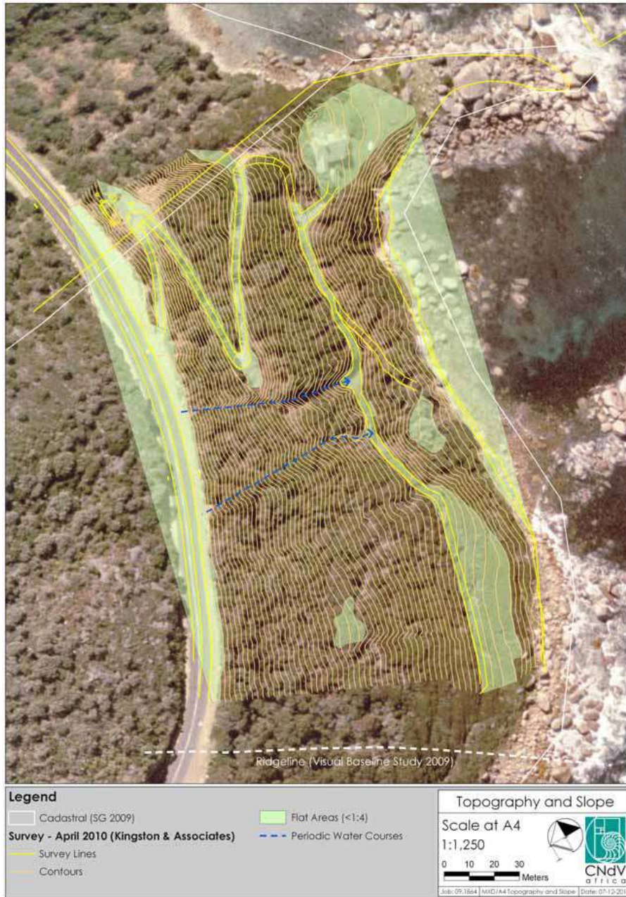
Fig 9. Topography of Partridge Point showing the steep slopes, the existing house on the promontory and a relatively level existing jeep track (c1:4) area along which the 3 cottages will be positioned. Not to scale: Source CNdV Africa.
