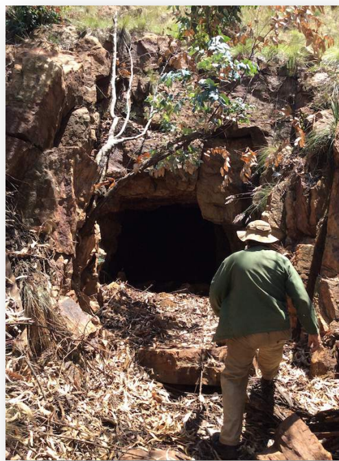
Figure 20 – Shallow incline shaft at RD05
