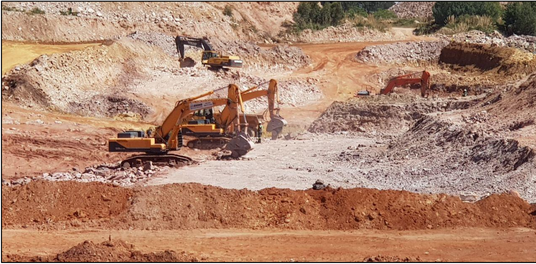
Figure 5: Closer view of the equipment used to break up the rock. The machine uses an Xcentric Ripper, which is an attachment developed for high-performance rock excavation and concrete demolition work. The production rates are up to 5 times greater than using a hydraulic breaker.
