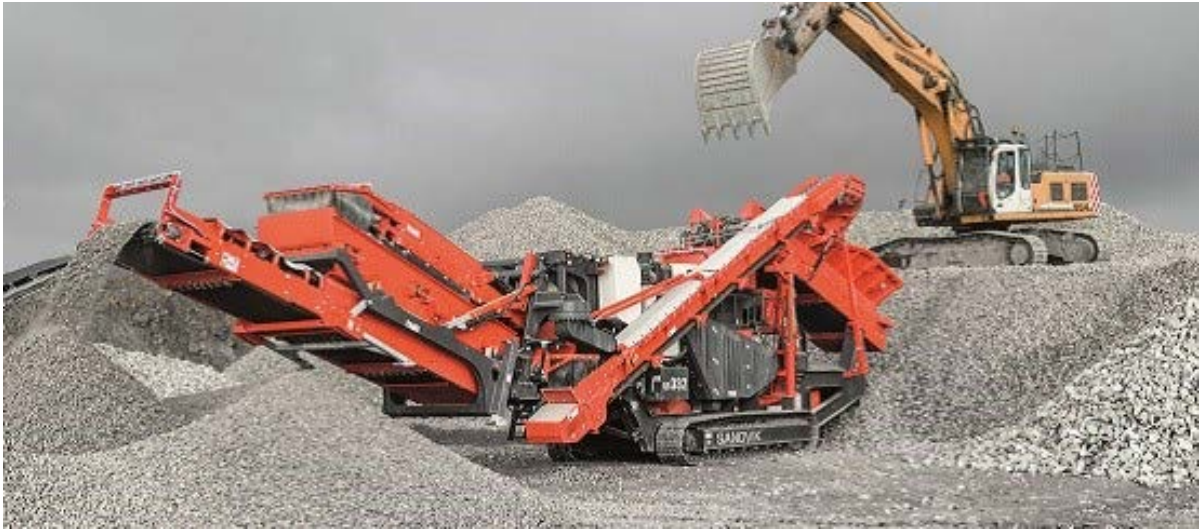
Figure 11. Typical example of a tracked mobile crush and screen plant.
