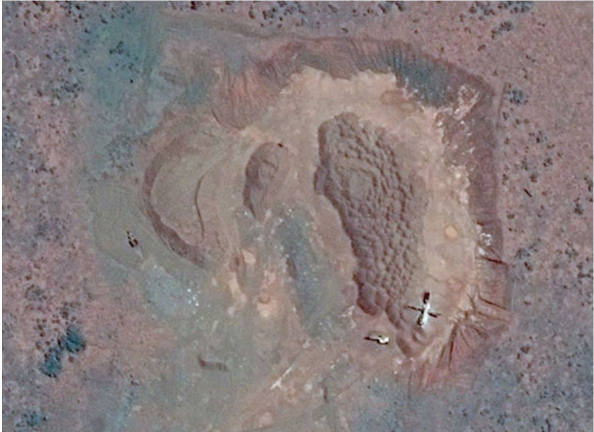
Figure 9. Google image from 2017. Note the presence of the mobile screen and crushing plant on the right, excavator below the plant and a dump truck to the left. Also note the extent and depth of excavations.
