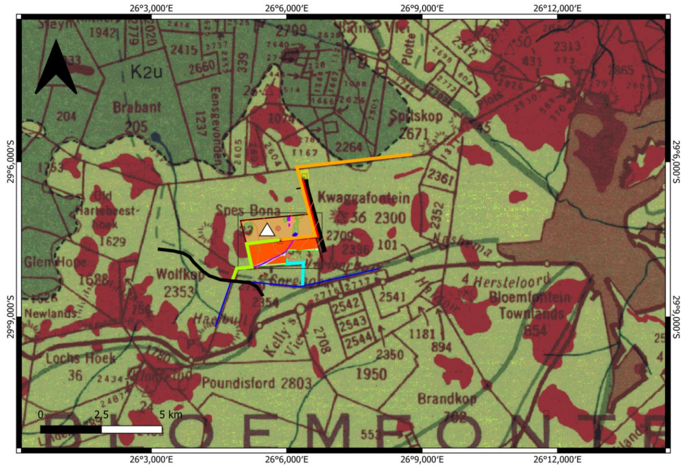
Figure 39: Extract of the 1:250 000 Bloemfontein 2926 Geological Map (1966) (Council of Geoscience, Pretoria) indicating the surface geology of the proposed development (indicated by the white triangle). The development is underlain by the Balfour Formation of the Adelaide Subgroup of the Karoo Supergroup.
