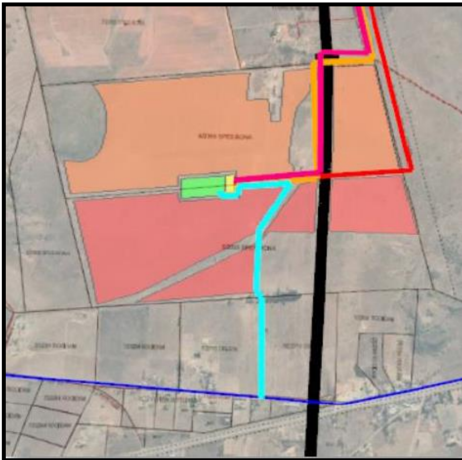
Figure 28: Planned connection from Bloemwater reticulation network to the operational centre of Harvard solar farm.
