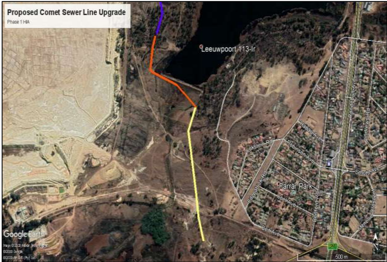
Figure 2: Section of the Sewer Line route close to Farrar Park & Cinderella Dam (Google Earth 2020).
