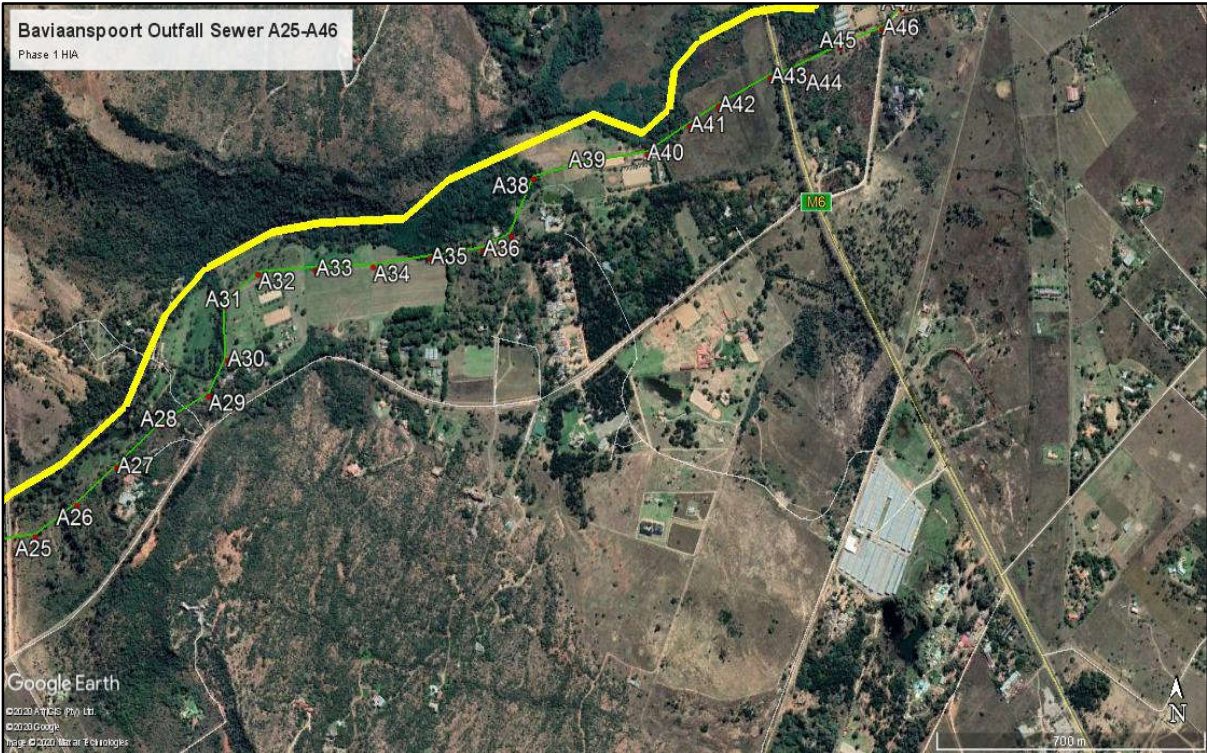
Figure 13: Aerial view showing Baviaanspoort line section from manhole point A25 up to A46 (Google Earth 2020).
