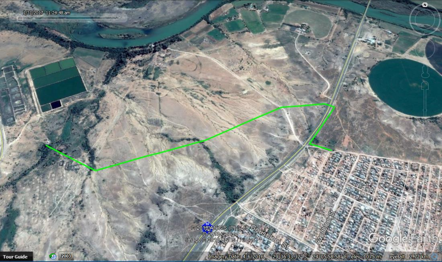
Figure 2: Google image indicating the proposed pipeline route in green, drainage lines to the orange river clearly visible.
