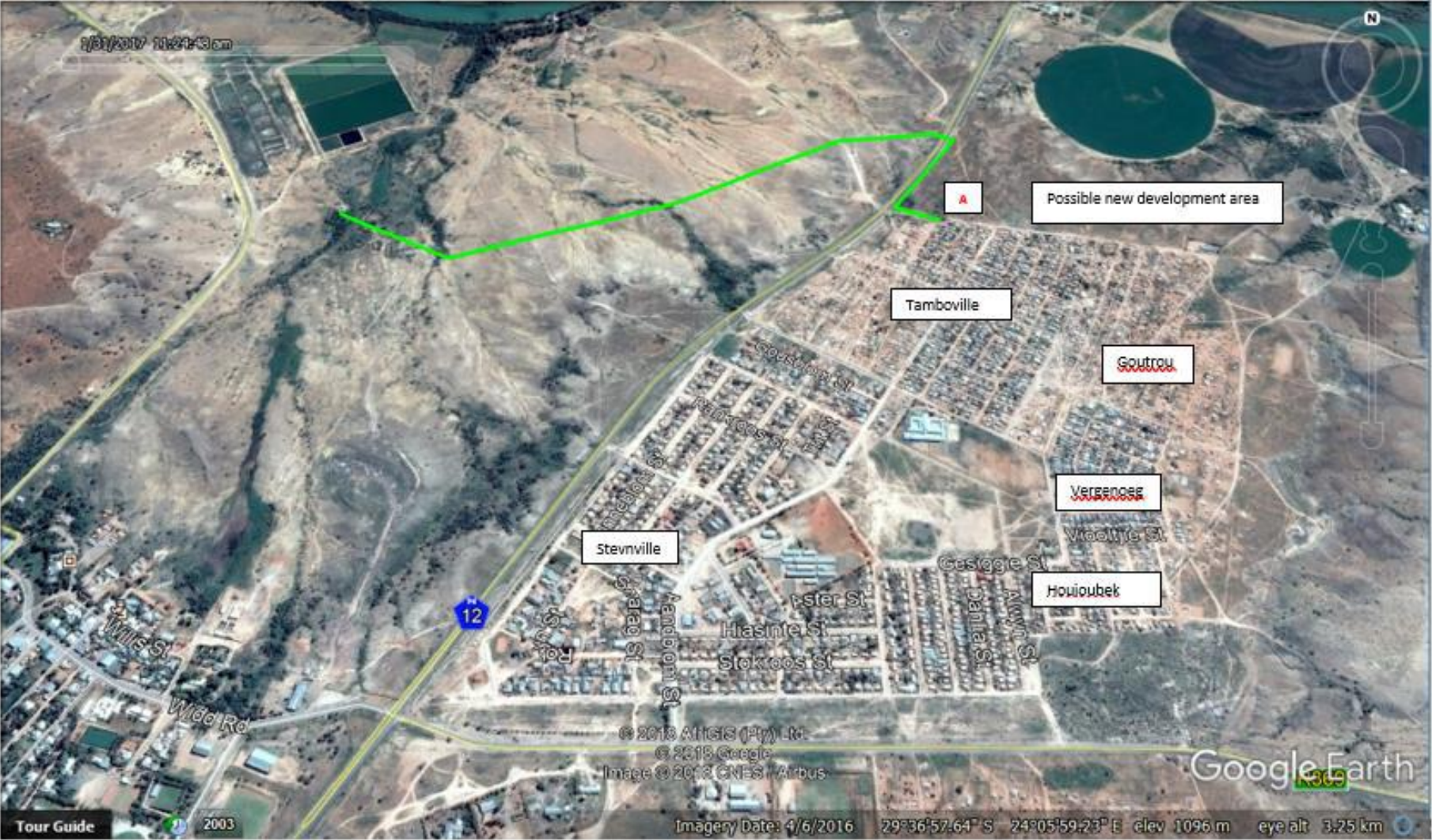
Figure 3: Google image indicating the proposed pipeline route in green as well as current suburbs and the possible new development area which will be serviced by the Hopetown Sewage Gravity Line/Outfall.
