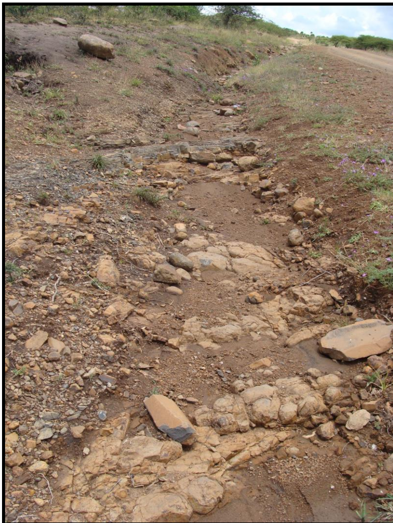
Figure 32: Stratigraphy exposed along the side of the road indicating dolerite in the foreground and shale sitting on top of siltstone in the background (GPS coordinates S 27° 53' 15.0" E 31° 50' 21.2")
