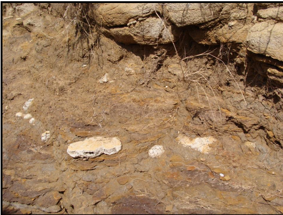
Figure 18: Zoomed in view of wall of roadside stratigraphy showing calcrete in shale (GPS co-ordinates S 27° 49' 07.02" E 31° 49' 59.70")
