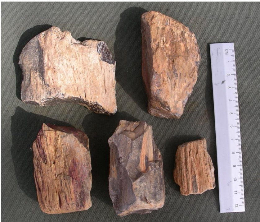
Figure 7: Transported fragments of silicified wood (hard so can survive being transported) from a Quaternary fluvial deposit.
