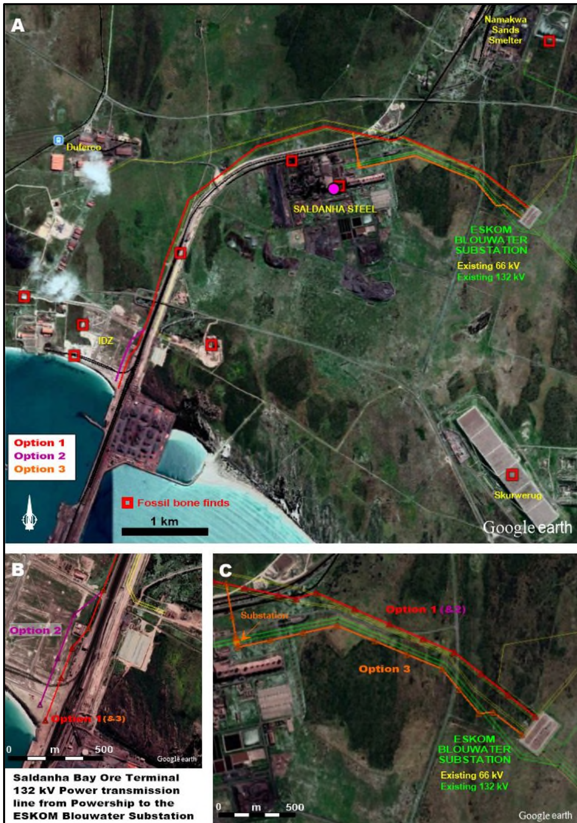
Figure 2. A: Proposed route options for the transmission lines. B: Detail showing Option 2 deviation from Option 1. C: Detail showing Option 3 deviation from Option 1.
