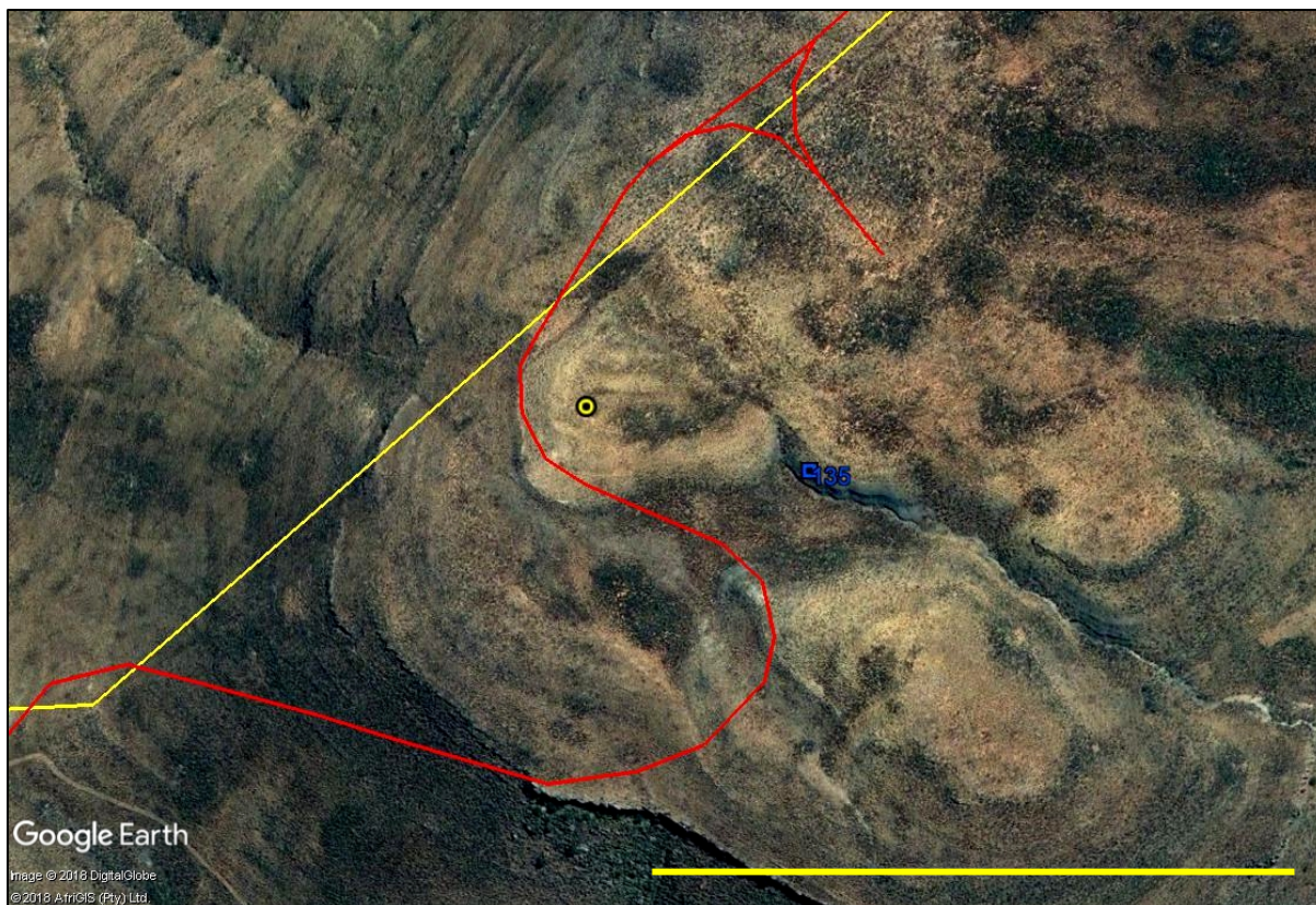
Figure 52. Close-up satellite image of fossil site Loc. 135 (assemblage of lungfish burrows within lacustrine mudrocks) situated close to the crest of the central turbine ridge on Gats Rivier 156. It lies in an erosion gully over 50 m from the nearest proposed access road (red) and wind turbine position (yellow dot) (Fig. 41) and is therefore unlikely to be impacted by the WEF development. Mitigation is therefore not proposed for this site. Scale bar = 300 m. N towards the top of the image.
