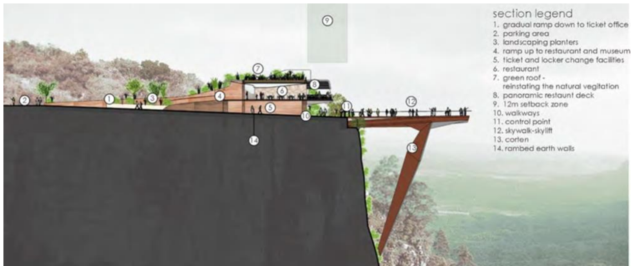
Figure 3: Artist's depiction of the side view of the proposed God's Window Skywalk construction. Supplied by Zutari.
