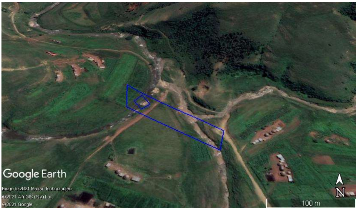
Figure 2: Google Earth map in more detail of the proposed culverts on L1526 with culvert 1 on the east (right) and culvert 2 on west (left), shown within the blue rectangle. Note that the route is along existing tracks and paths and crosses the Nxway River. Map supplied by Gedezar Consulting.
