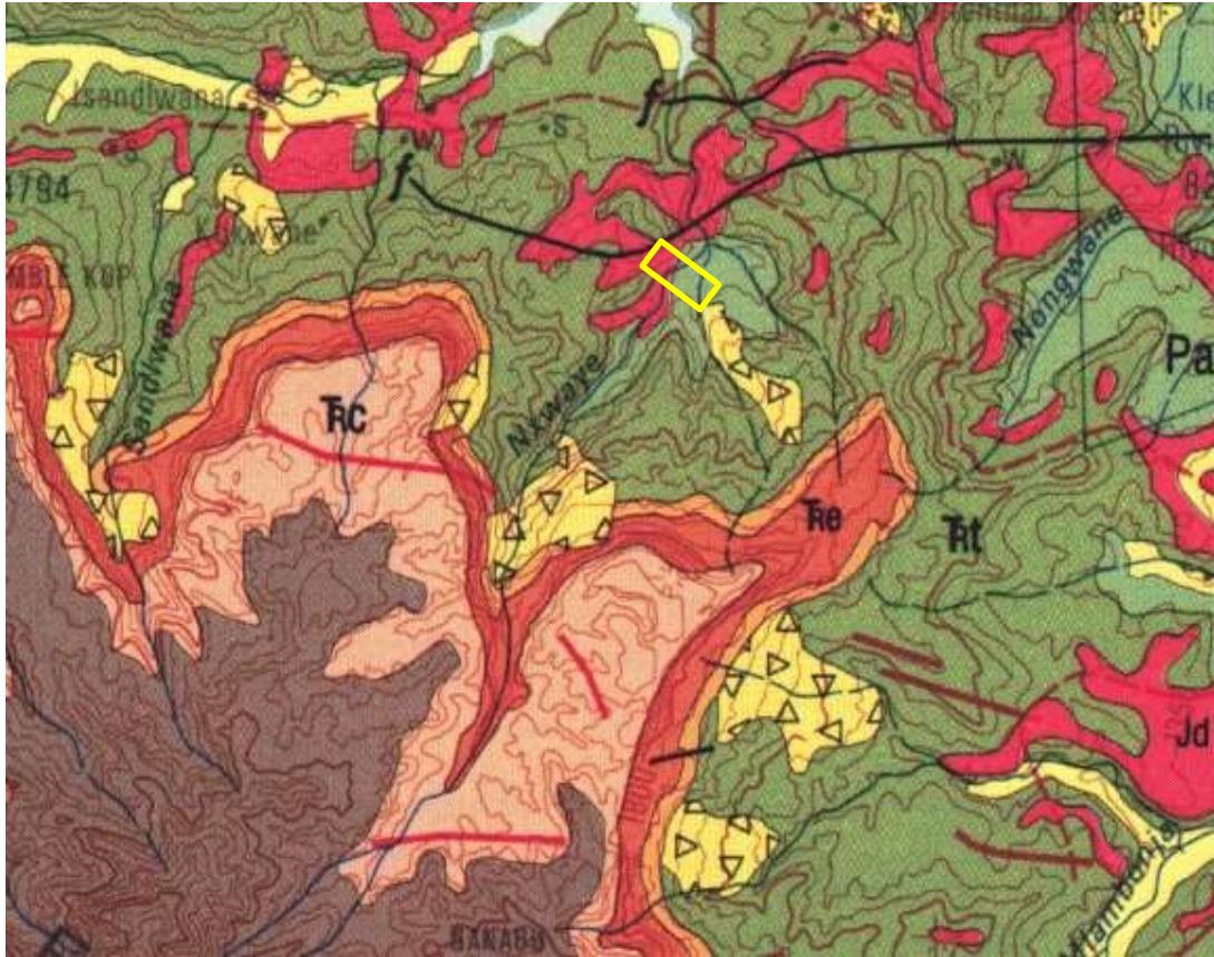
Figure 3: Geological map of the area around the proposed L1526 culverts over the Nxwaye River. The location of the proposed project is indicated within the yellow rectangle. Abbreviations of the rock types are explained in Table 2. Map enlarged from the Geological Survey 1: 250 000 map 2828 Harrismith.
