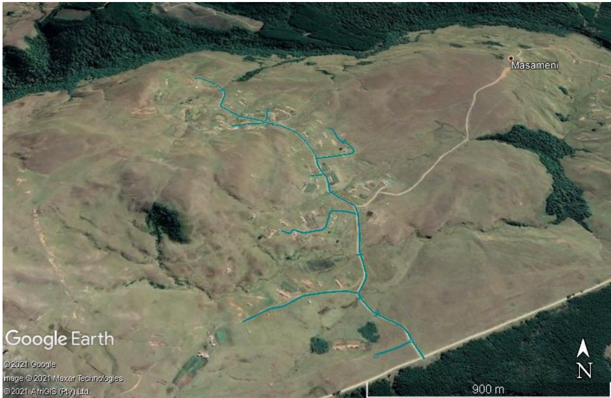
Figure 2: Google Earth map in more detail of the proposed access road through Zamazela, shown by the blue line. Note that the route is along existing tracks and paths. Map supplied by Greenbelt.
