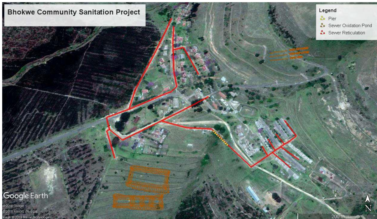
Figure 1: Google Earth map of the proposed upgrading of the sanitation system in Bhokwe Village, Bhokwe Community, Ward 05, AbaQulusi Municipality. The red lines indicate the sewer reticulation and the orange lines show the sewer oxidation ponds.
