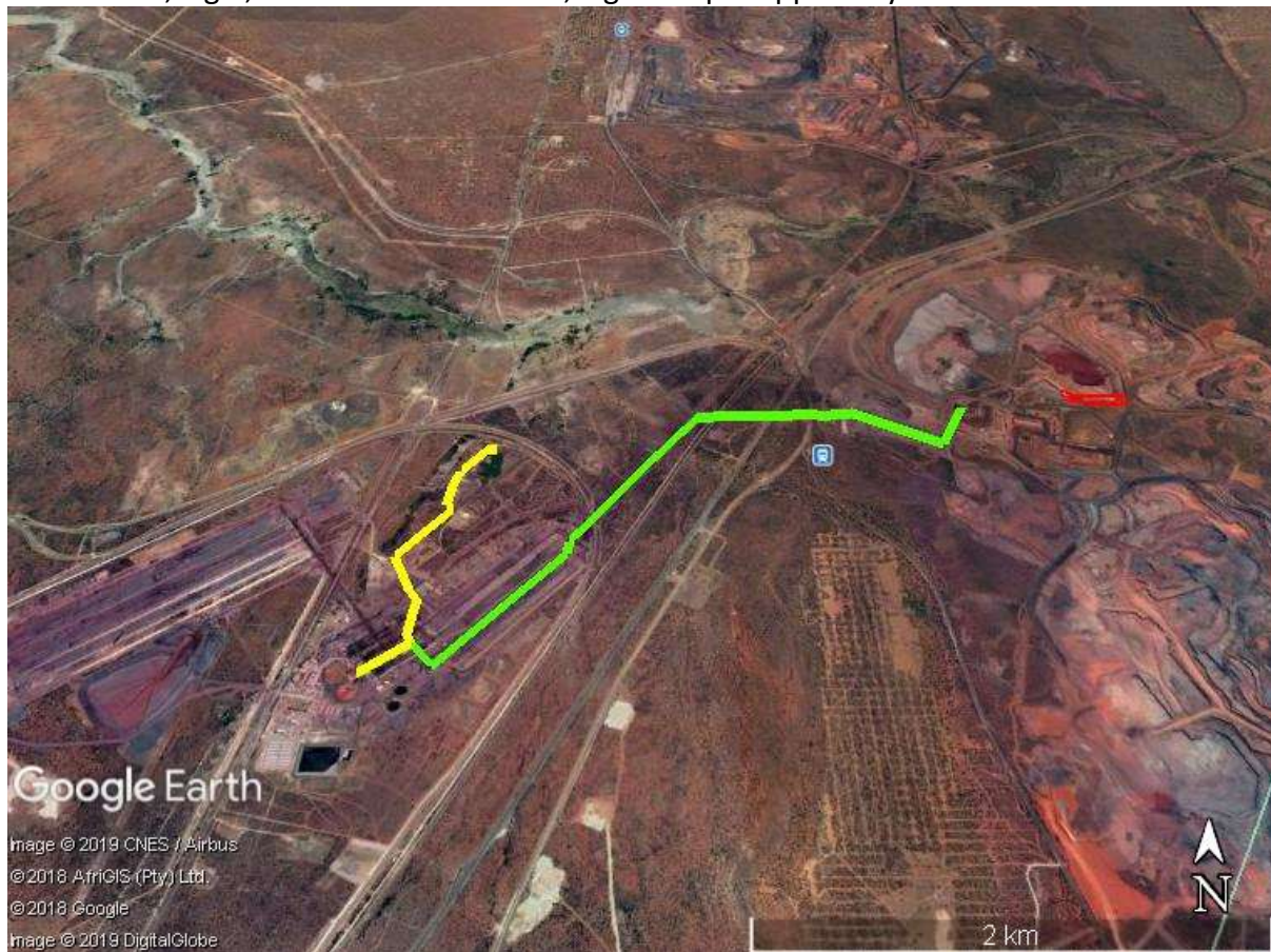
Fig. 2; Green = Waste Disposal Facility return water pipeline, Fig. 2; Red = proposed Slimes Water Dam, Fig 3; Blue = water reservoir, Fig 4. Maps supplied by HCACA.
