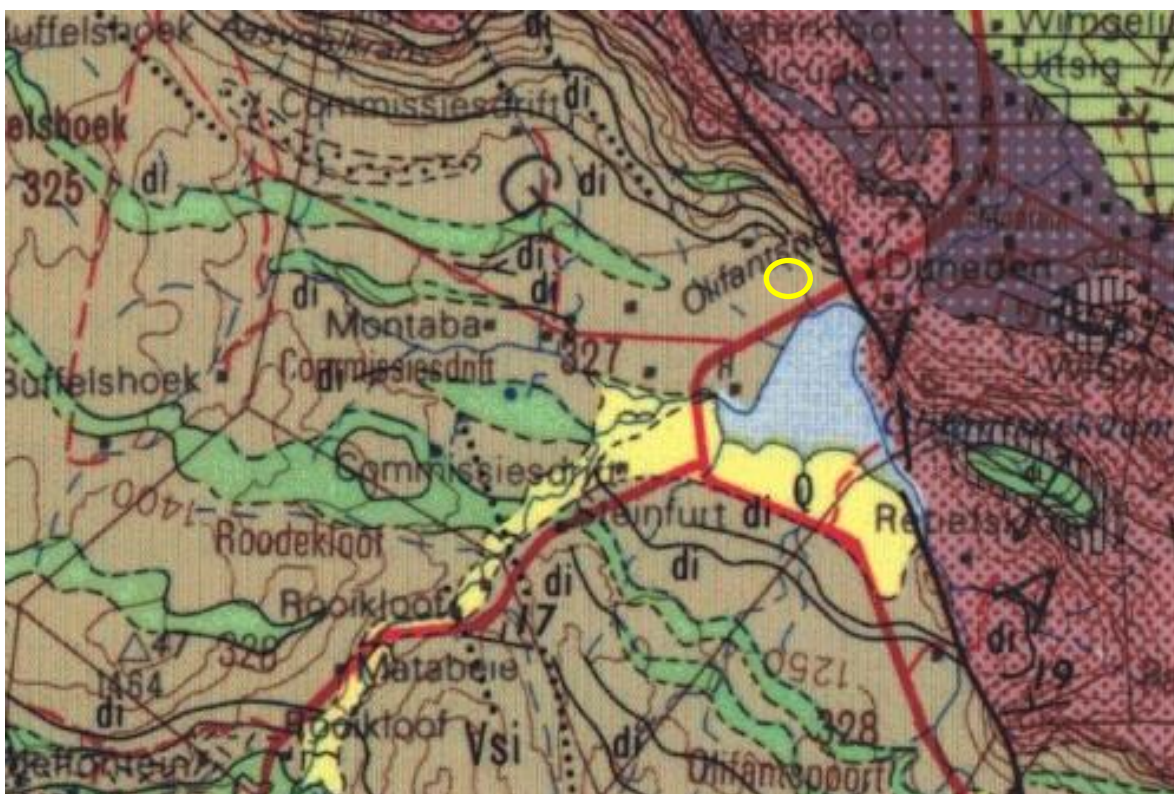
Figure 2: Geological map of the area around the Farm Commissiesdrift 327 JQ with the proposed site for the Olifantsnek Vodacom mast shown within the yellow outline on rocks of the Silverton Formation (symbol Vsi, grey). Abbreviations of the rock types are explained in Table 2. Map enlarged from the Geological Survey 1: 250 000 map 2526 Rustenburg.
