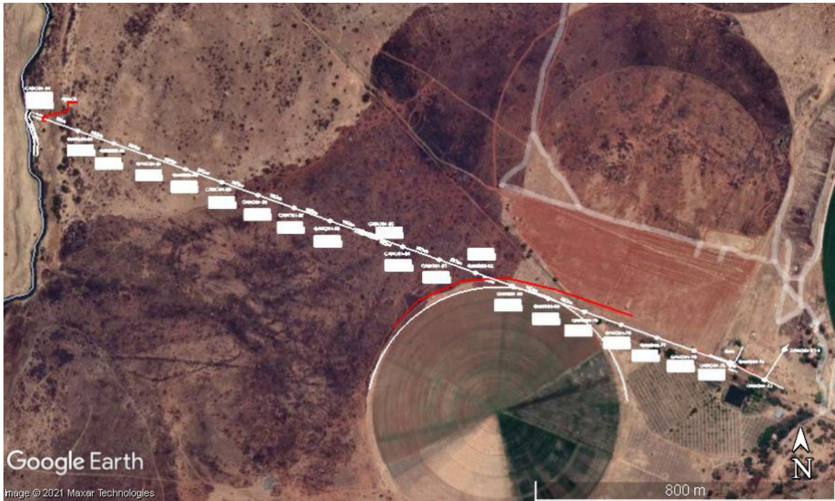
Figure 2: Google Earth map to show the proposed route (and pole type) for the 22 kV powerline south of Pampierstad, Northern Cape Province.
