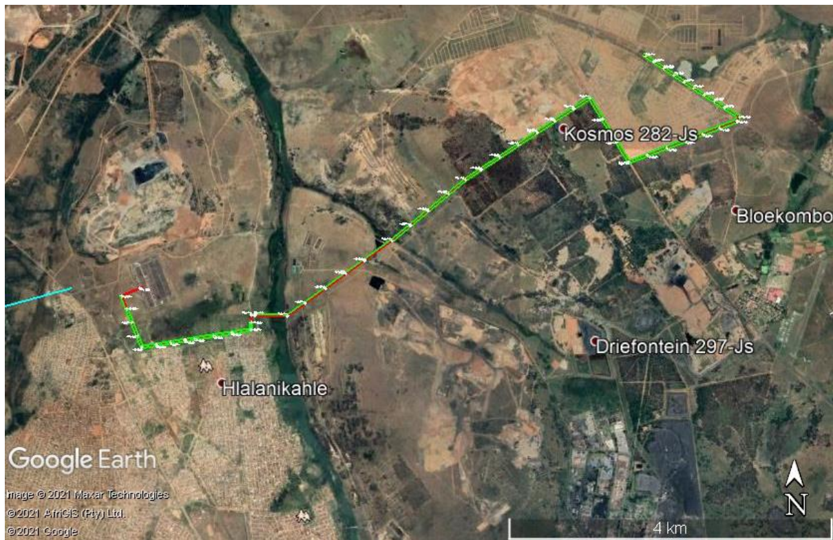
Figure 1: Google Earth map of the proposed route for the Siyanqoba 132kV Overhead Electrical Line with the sections shown by the green line outline. Map reference: 1.VE2001-1-RP REVC 2020-04-15.
