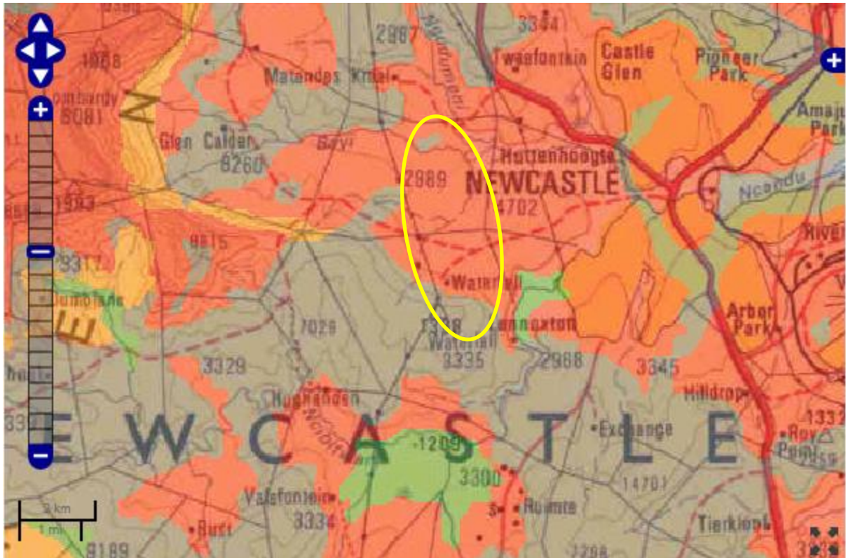
Figure 4: SAHRIS palaeosensitivity map for the site for the proposed mining right on Farms Craig and Waterfall for the Newcastle Project shown within the yellow rectangle. Background colours indicate the following degrees of sensitivity: red = very highly sensitive; orange/yellow = high; green = moderate; blue = low; grey = insignificant/zero.
