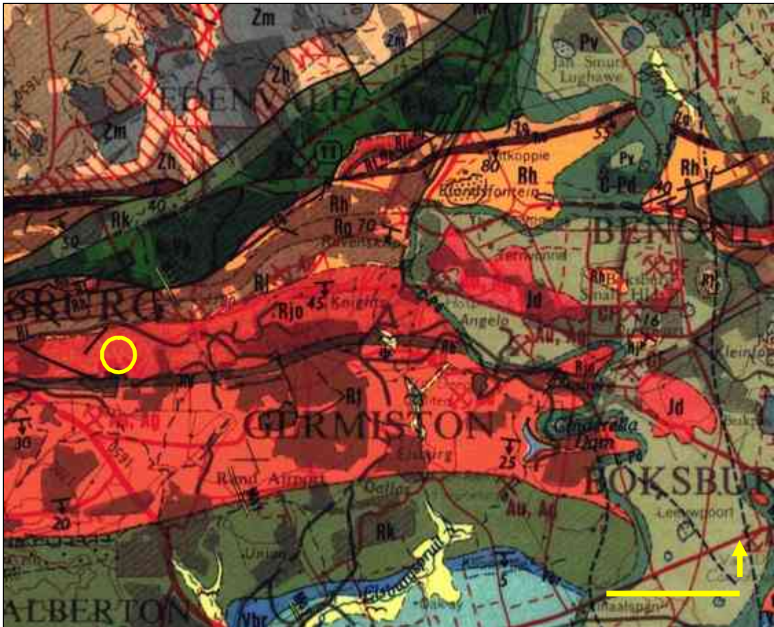
Figure 1. Extract from 1: 250 000 geology sheet 2628 East Rand (Council for Geoscience, Pretoria) showing the approximate location of the Jupiter Extension 9 study site (yellow circle). The site is largely underlain by south-dipping fluvial quartzites of the Johannesburg Subgroup (Central Rand Group, Witwatersrand Supergroup) of Archaean age (Rjo, red) as well as reworked mine tailings at surface. Scale bar = 4 km. Arrow points to North.
