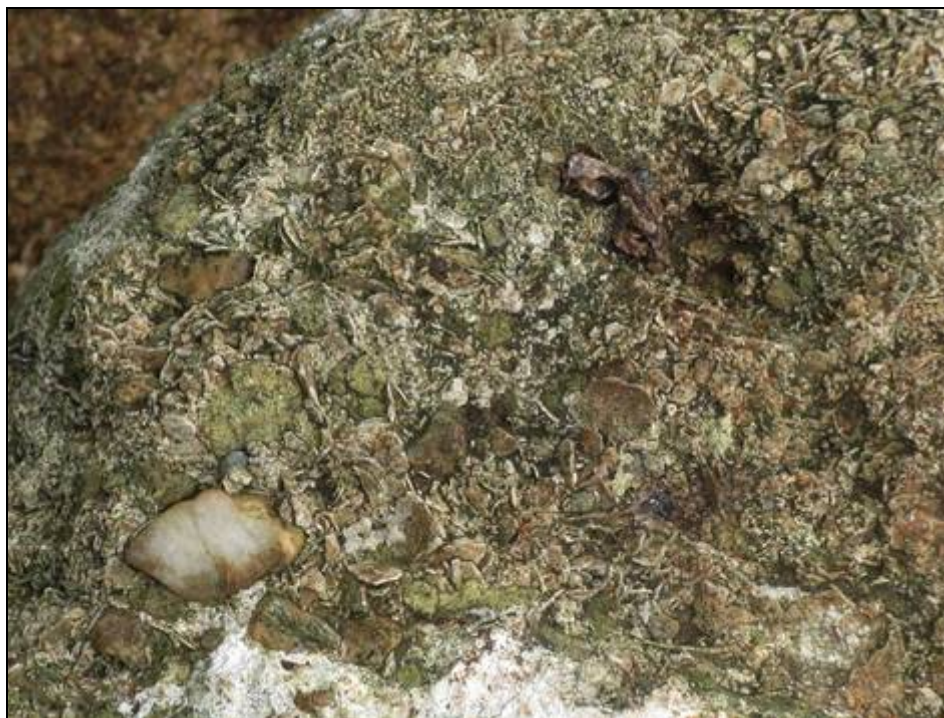
Fig. 20. Close up of float block of Bathurst shelly limestone or coquinite showing mass of small shell fragments (shell hash) and small pebbles. The largest pebble here is c. 1 cm across.
