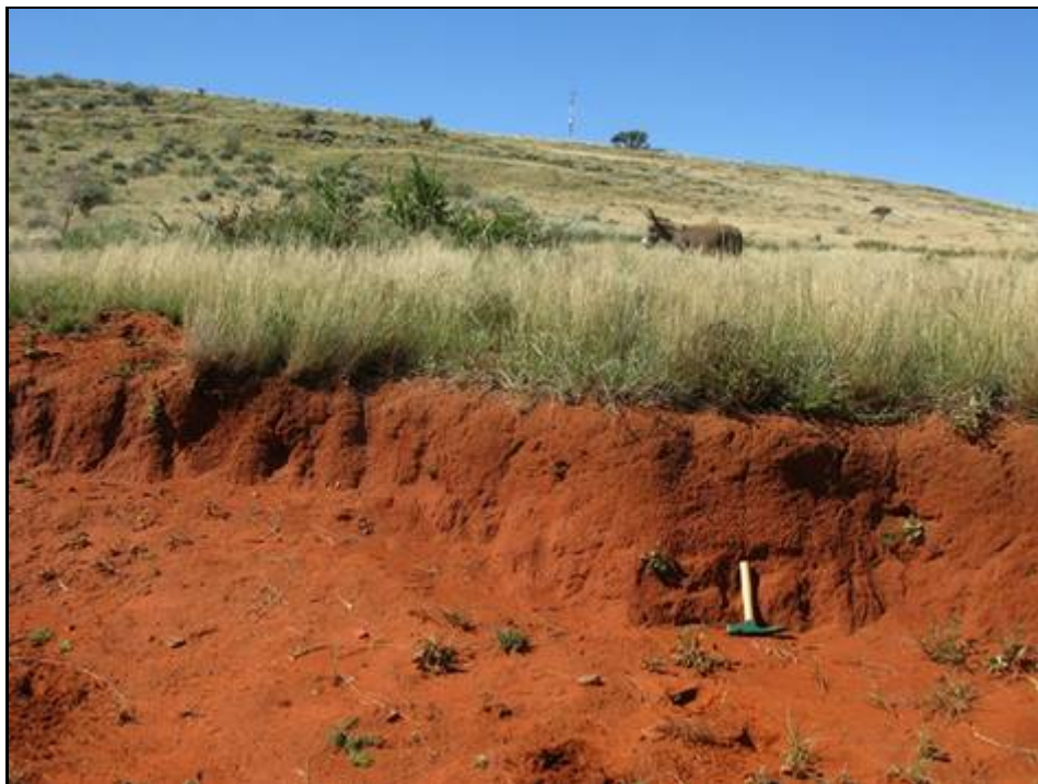
Fig. 17. Borrow pit into typical orange-brown Kalahari sands of the Gordonia Formation at Metsimetala Village (Loc. 504) (Hammer = 27 cm). The hillslope behind is built of Ongeluk Formation lavas.
