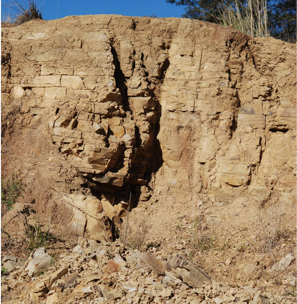
Figure 9. Borrow pit 049 BP03 near Kentani exhibiting finely laminated grey to yellow sandstone.
