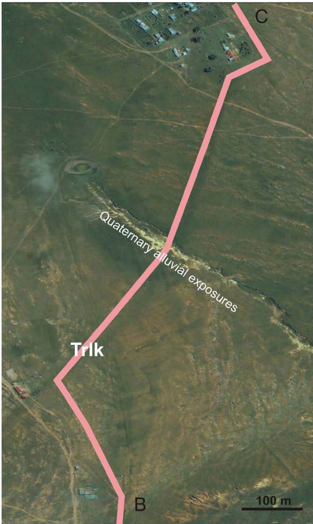
Figure 8. Gravity Main. Aerial view of Section B - C. The section is underlain by fossil-bearing Katberg Formation sandstone ( Trlk ) and substantial superficial valley fill deposits of Quaternary age.
