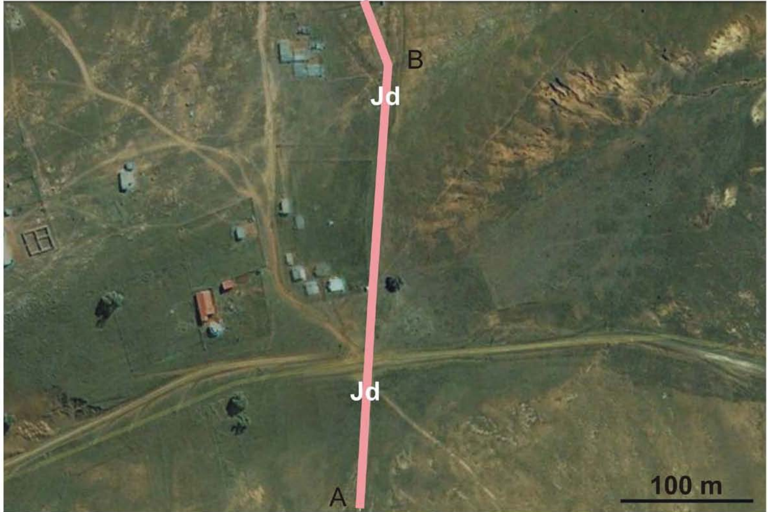
Figure 6. Gravity Main. Aerial view of Section A - B. The section crosses approximately 300m of interconnected dolerite intrusions and superficial Quaternary-age valley deposits.
