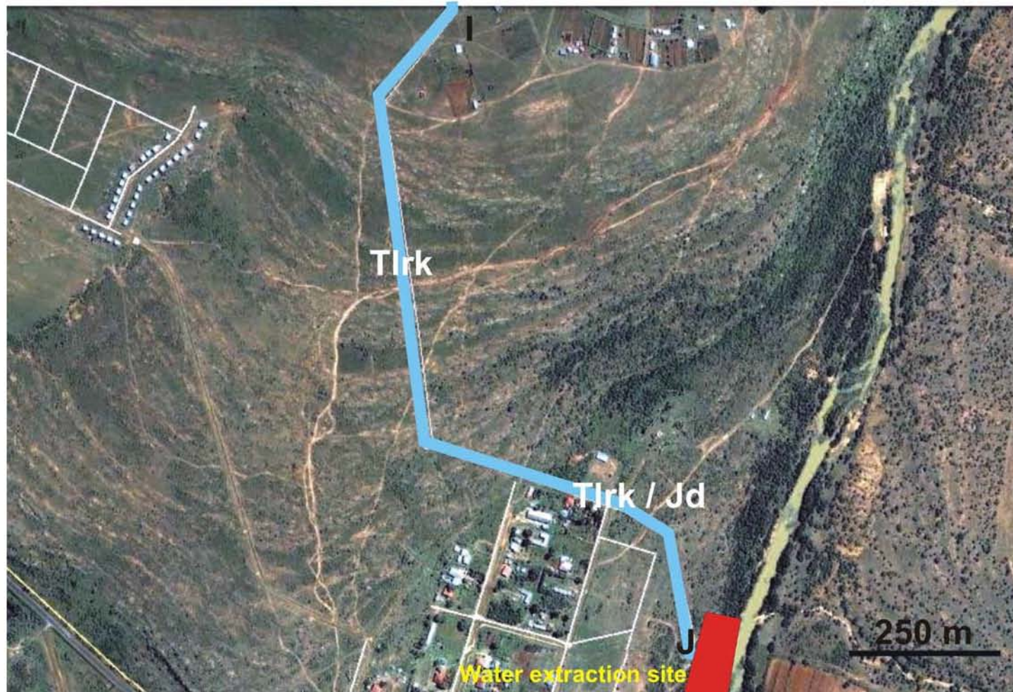
Figure 17. Pumping Main. Aerial view of Section I - J. The section is underlain by fossil-bearing Katberg Formation sandstone ( Trlk ). Dolerite intrusions are also widespread along the upper terrace of the Tsomo River at the current water extraction site.
