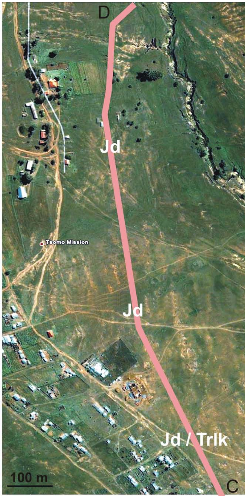
Figure 10. Gravity Main. Aerial view of Section C - D. The underlying geology is mostly made up of dolerite bedrock ( Jd ) and Quaternary alluvial sediments.
