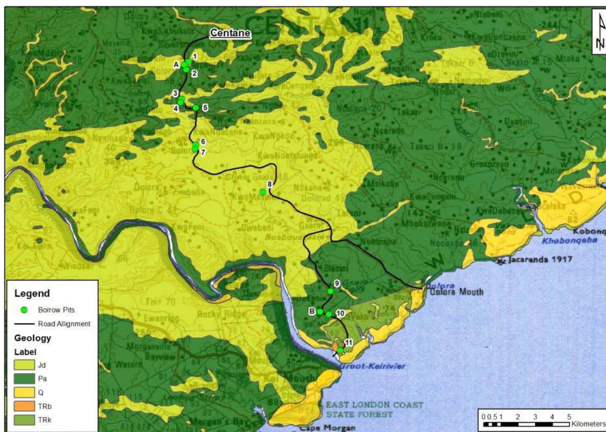
Figure 1. Geological map of the study area showing the positions of borrow pits (1-11) as well as other areas of interest. Pa = Adelaide Subgroup, TRk = Katberg Formation (Tarkastad Subgroup), TRb = Burgersdorp Formation (Tarkastad Subgroup), Jd = dolerite, Q = Quaternary cover
