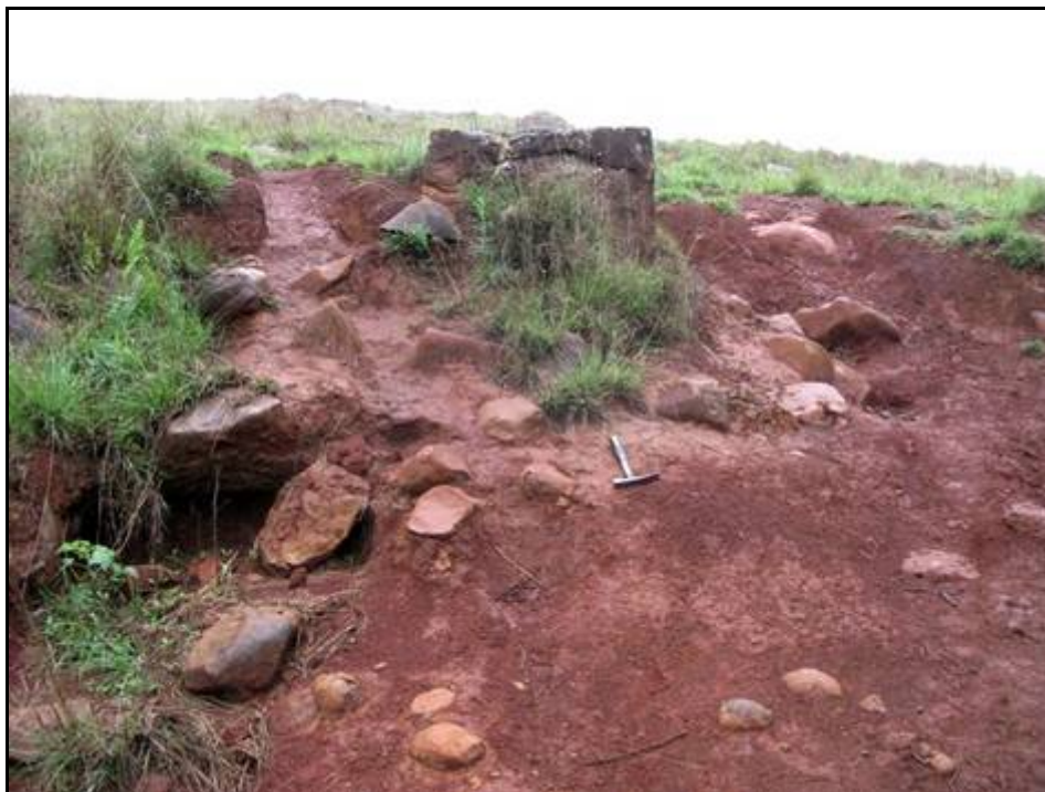
Fig. 5. Reddish-brown ferruginous soils overlying weathered dolerite, with floating dolerite corestones, north-western outskirts of Cenyu village (Hammer = 30 cm).
