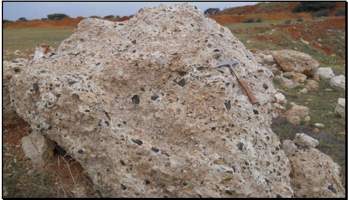
Figure 3.3 Conglomerate with poorly rounded pebbles of mainly Ongeluk lava in the calcareous Kalahari Formation
