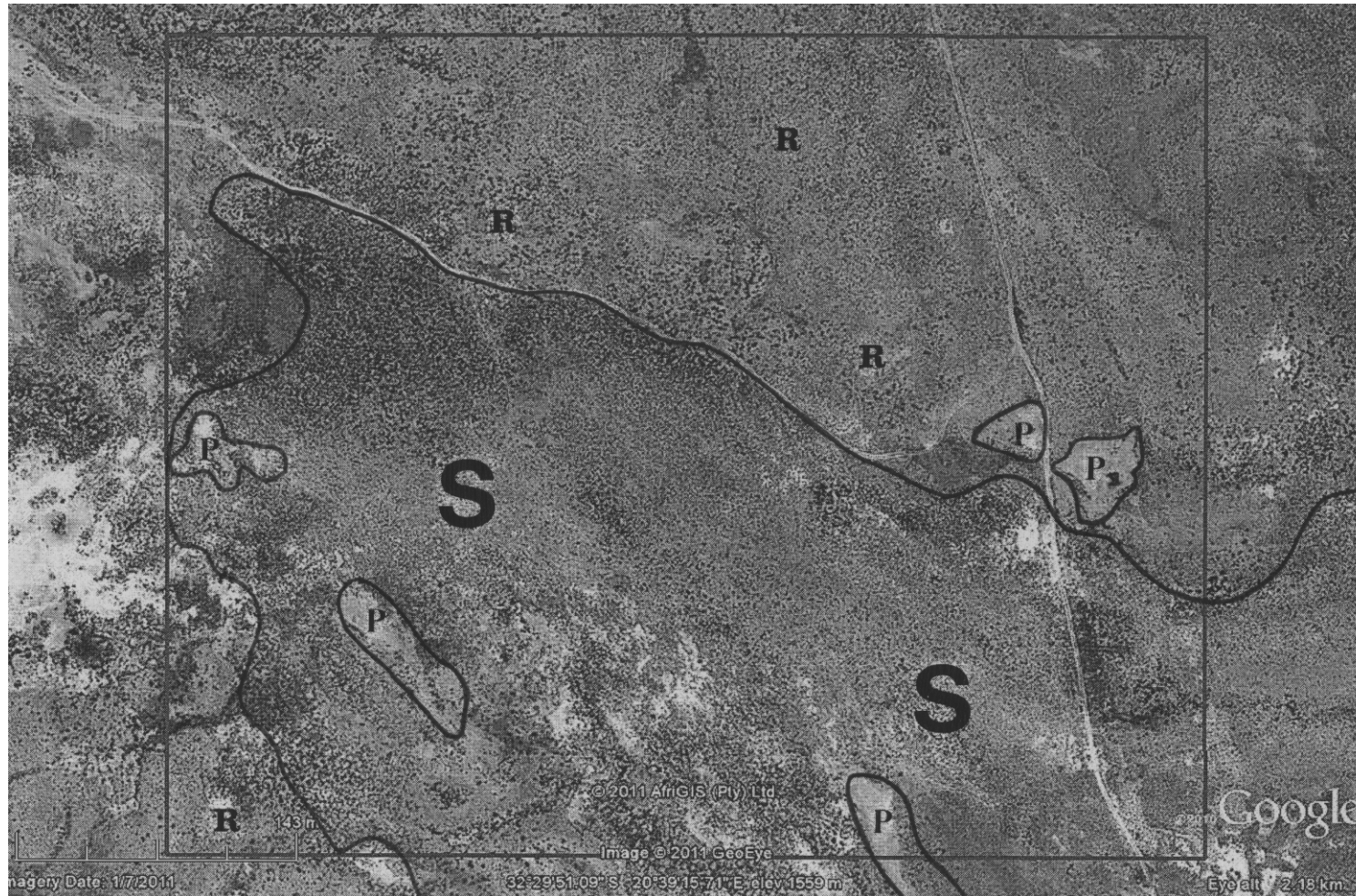
FIGURE 5: REVISED DEVELOPMENT SITE: OPTION 1 R = Rock sheets, exposed rock, rocky ridges. P = Pans. S = Sandy area suitable for solar development.
