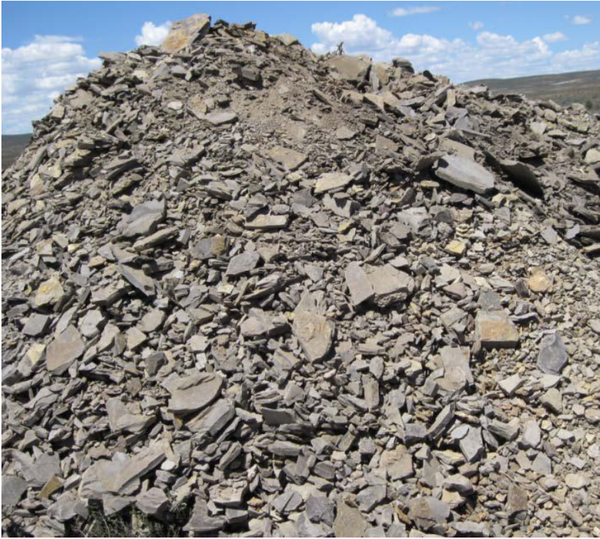
Fig. 6. Pale grey shales of the Whitehill Formation excavated from trial pit TP6 in the north-central part of the study area (see Fig. 2). Coherent, moderately weathered mudrocks of this sort may still contain fossil material such as remains of fish, reptiles and crustaceans. Image abstracted from the geotechnical report by Mainstream Renewable Power (Anon, 2011).
