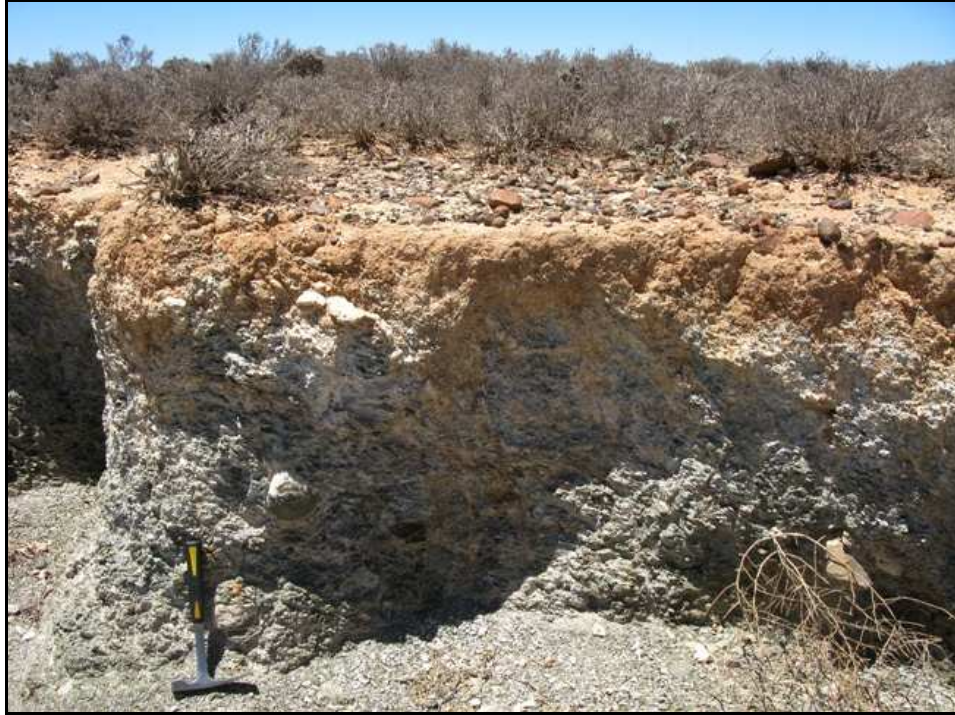
Fig. 13. Downwasted surface gravels overlying thin orange-brown soils and deeply-weathered, calcretised Dwyka boulder mudstones, Quarry 1 (Loc. 306) (Hammer = 30 cm).
